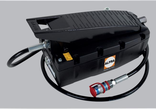
Air-hydraulic pump for the operation of single-action hydraulic cylinders for whole punchers, cable cutters, presses or similar applications.
